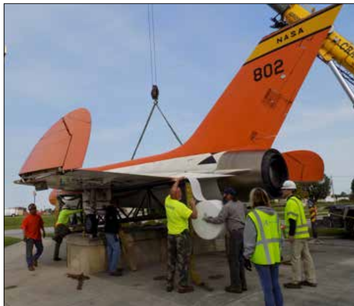
The moving team, including Thomarios and ICA, slid ethafoam between the frame and the Skylancer's wing to provide padding for the wings and prevent any possible abrasions from the support frame.
